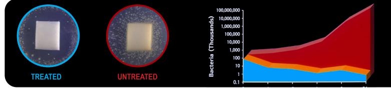
These samples were tested for efficacy against bacteria. The left sample was manufactured with our antimicrobial additive, the sample on the right was not. Both samples were inoculated with bacteria and then photographed after 24 hours. The sample with antimicrobial proptection shows no growth while the unprotected sample shows significant contamination.
